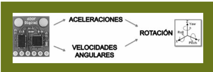
Figura 6. IMU Digital Combo Board 6 Degrees of Freedom de Sparkfun
